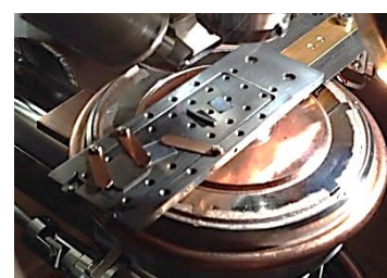
Turn the magnetic ring and pull it out.
