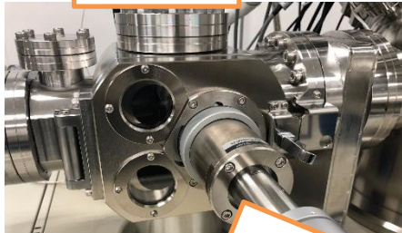
When evacuate, push the vessel body in a little by hand.
