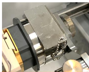
Ensure the chain does not get tangled when attaching the observation window cover.
