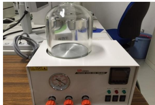
Vacuum heating/deaeration system
